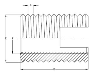
Female thread A = M6Length B = 10Male thread E = 8.0Min hole depth blind hole = 13Recommended bore diameter (hard mat.) = 7.3 to 7.5Recommended bore diameter (soft mat.) = 7.1 to 7.2Thread pitch P = 1.00Type  $= 303 \ 0 \ 060$ .
